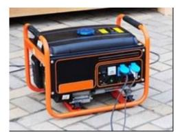
They should not be used inside any building and ideally should be placed some distance away from a property. However, we have heard of instances where generators have been in garages or too close to the house and CO has blown in via vents sometimes setting off the CO alarms in the property.
